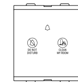
DND-MMR: OUT-SIDE ROOM UNIT
